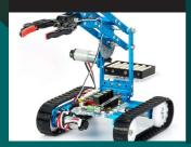
Ultimate 2.0 is a flagship robot kit based on Makeblock platform with rich features and strong compatibility. It helps learn about mechanical structure, electronic modules and programming.
